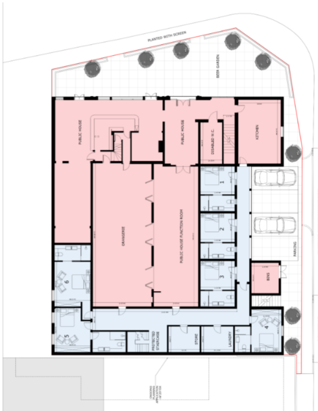
Proposed Ground Floor Plan (Floorspace shown in pink would be pub use, floorspace shown in blue would be hotel use and the existing building at no.10 Eaton Place is shown in grey in the top left-hand corner)
